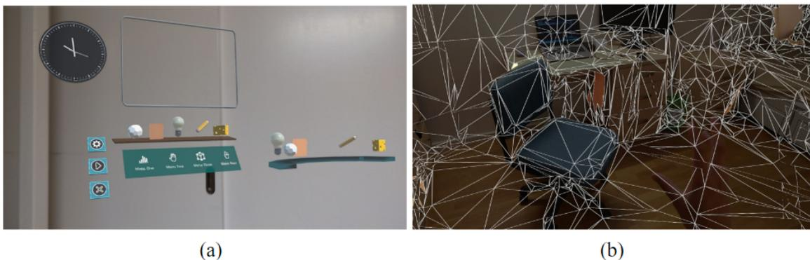
Fig. 1.2 (a) A sample UI designed for the HoloLens 2 using Unity, (b) the spatial mapping feature of the device.
